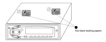
There are 2 mounting screws on the case of the DVD player( as above figure shows) to protect the unit during shipping.
